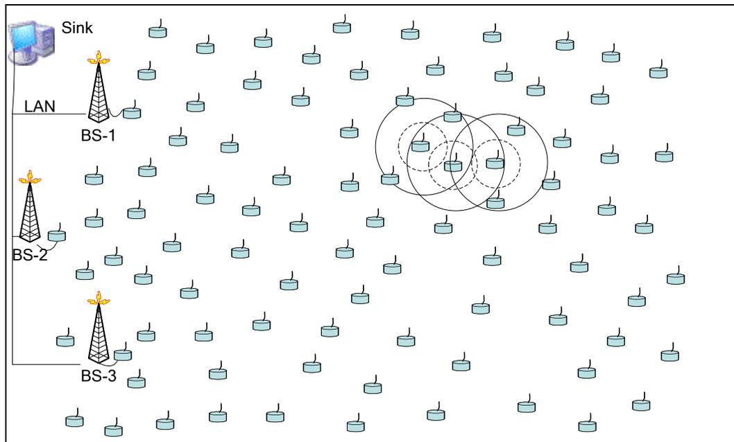
**Fig. 1.** A typical sensor theater. Three base stations organized as an equilateral triangle and a single sink monitor the wireless sensor network.
