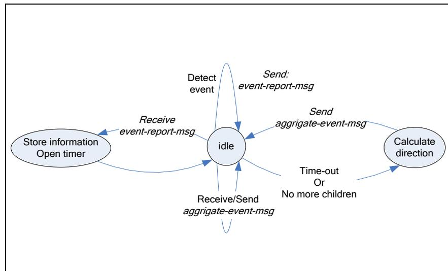
Fig. 4. node basic automaton
